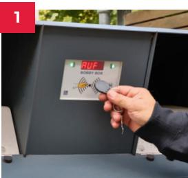
Hold the transponder (chip) in front of the transponder panel. The green indicator lights up and the compartments are unlocked.
